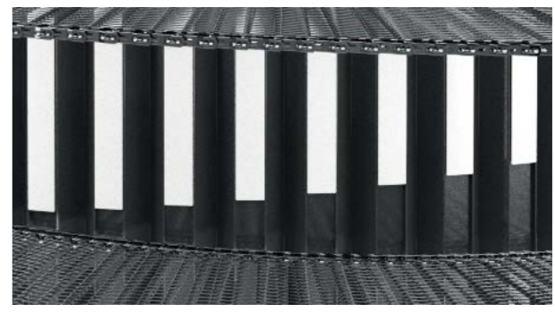
REMOVE THE FLAT LOW TENSION CAGE BARS
