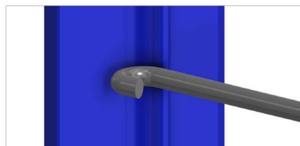
OPTIMAL CONTACT AREA DUE TO THE ROUND TOOTH AND BENDED ROD
