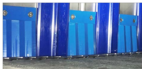
END OF THE CONICAL BLOCK IN THE BOTTOM PART OF THE DRUM
