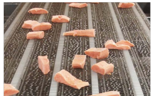
Wire mesh belt used to transport salmon.
