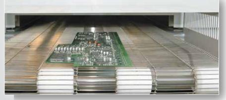
Wire mesh belt used in soldering furnace.
