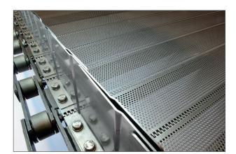
Perforated plate belts are well suited for a.o. drying processes. Their self-supporting structure means they can be used over large widths without additional support.
